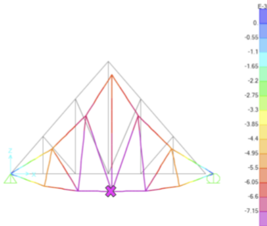
Figure 3a. Maximum deflection of the higher sloped, 24 foot Howe truss occurs at the points marked by the pink Xs and is a downward deflection of 0.0902 inches.
