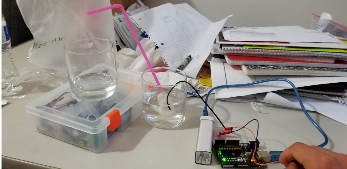
Figure 11: Pump testing using Arduino Uno
